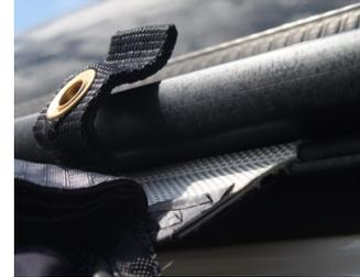
2. Slide the awning piping through the awning channel, until the awning is in the desired position on the vehicle; we suggest having someone else hold the canvas in position whilst you do this.
