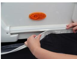
9. Thread the draught skirt through the lower awning channel and secure it at each side using groundsheet pegs.
