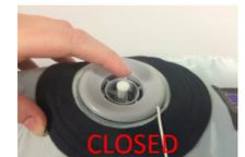
6. Begin inflating the Oxygen Air Frame, until you can give it a 'good squeeze', as the tube requires space for air to expand, in case of a fluctuation in the ambient temperature. Do not concern yourself about overinflation, however, as the pressure relief valve expels excess air above 6PSI.
